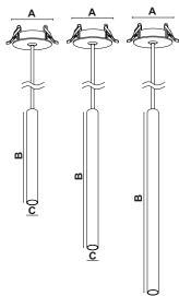
Suitable for Ceiling thickness 5-20mm.
